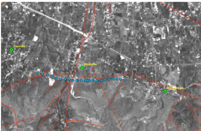
**Fig. 9** SPOT4 satellite orthorectified image (PAN) of the area of Mournies, showing the path (blue dots), along which VLF measurements were obtained. The red lines indicate the location of the fault features represented at the IGME map.
