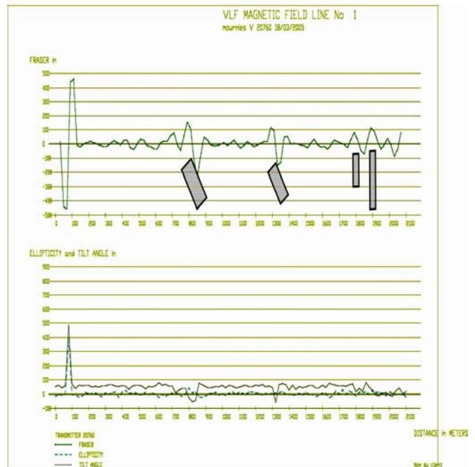
**Fig. 10** Results of the VLF measurements conducted in the area of Mournies, close to the public hospital of Chania (bottom). Source frequency was equal to 20.7 kHz. X-axis represents the distance from the beginning of the profile. The Fraser filtered data, together with the measurements of ellipticity and tilt angle are given in the graph above (top).
