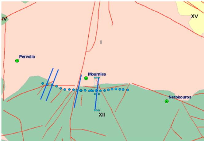
**Fig. 11** Map of the morphometric units outlined in the area of Fig. 9. There is a clear relation between the tectonic features defined in the geological map (red lines) and the fractures located by the VLF measurements (blue lines). The direction of the fractures at the specific locations is shown on Fig. 10.
