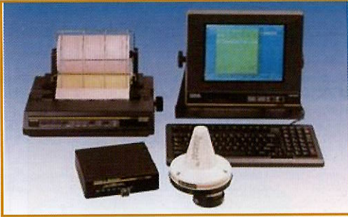
Fig.4 Hardware components of a typical INMARSAT-C terminal
