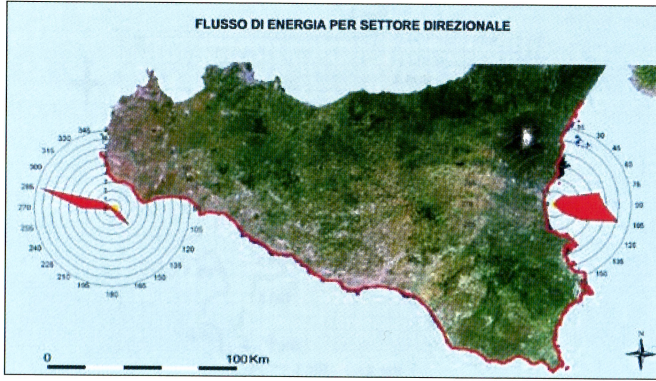
Figure 8 Radar plot of energy flux –Coastal sector C6: Marsala – C.po S. Alessio
